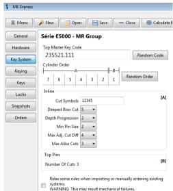
This screen changes depending on the System type you are using. These are the rules that are used when calculating a Master Key system...
