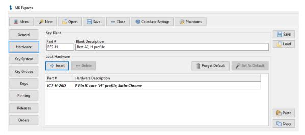
When creating an order, MK Express records the hardware selected for each cylinder/lock. So upfront it needs to know what part numbers are going to be used. This screen allows you to list the part numbers and descriptions of the hardware you'll be installing.
